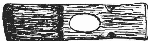
GT 1198 Copper hammer, flat square face with straight pane.
