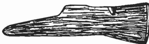
GT 1242 Iron hammer, flat square face with cross pane, similar to French pattern hammer, Salaman (1975).
