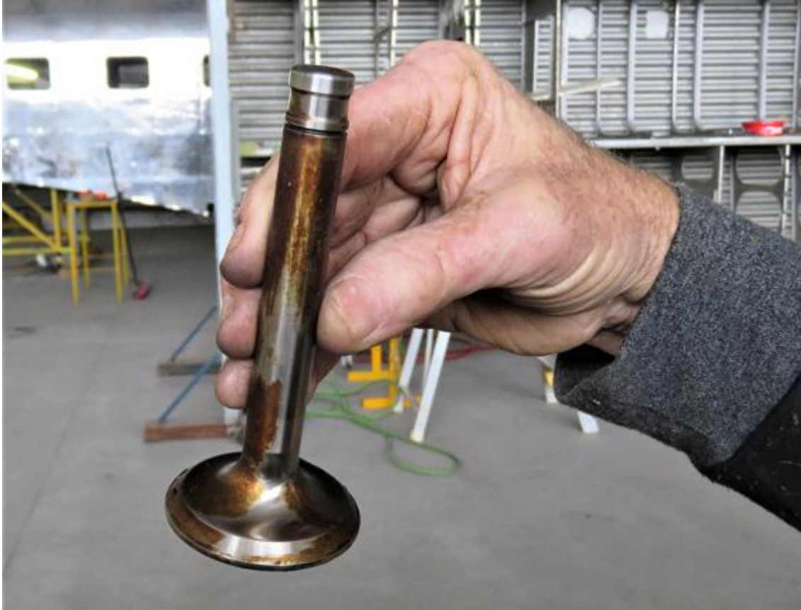
A valve from the DC-2 engine, five metals welded together.
