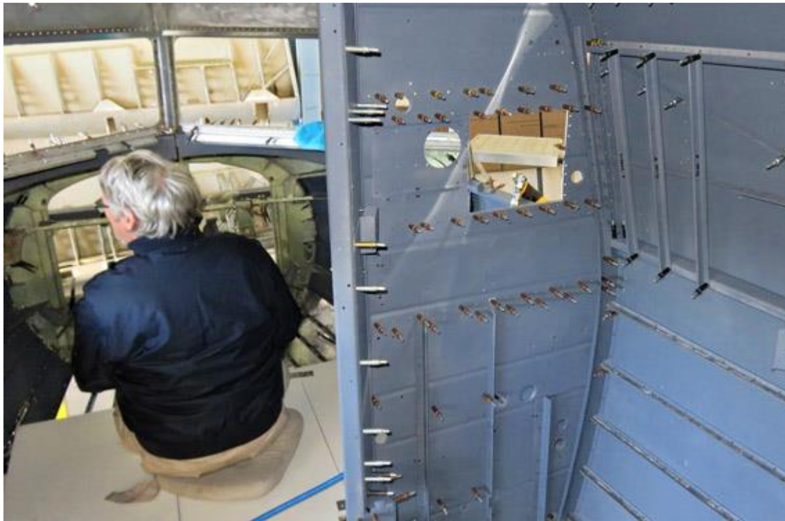
The new bulkhead helps to give shape to the DC-2 cockpit.
