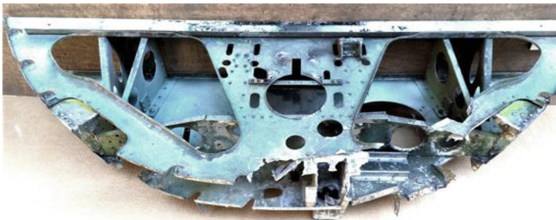
The damaged yoke mounting that was taken out of the aircraft...
