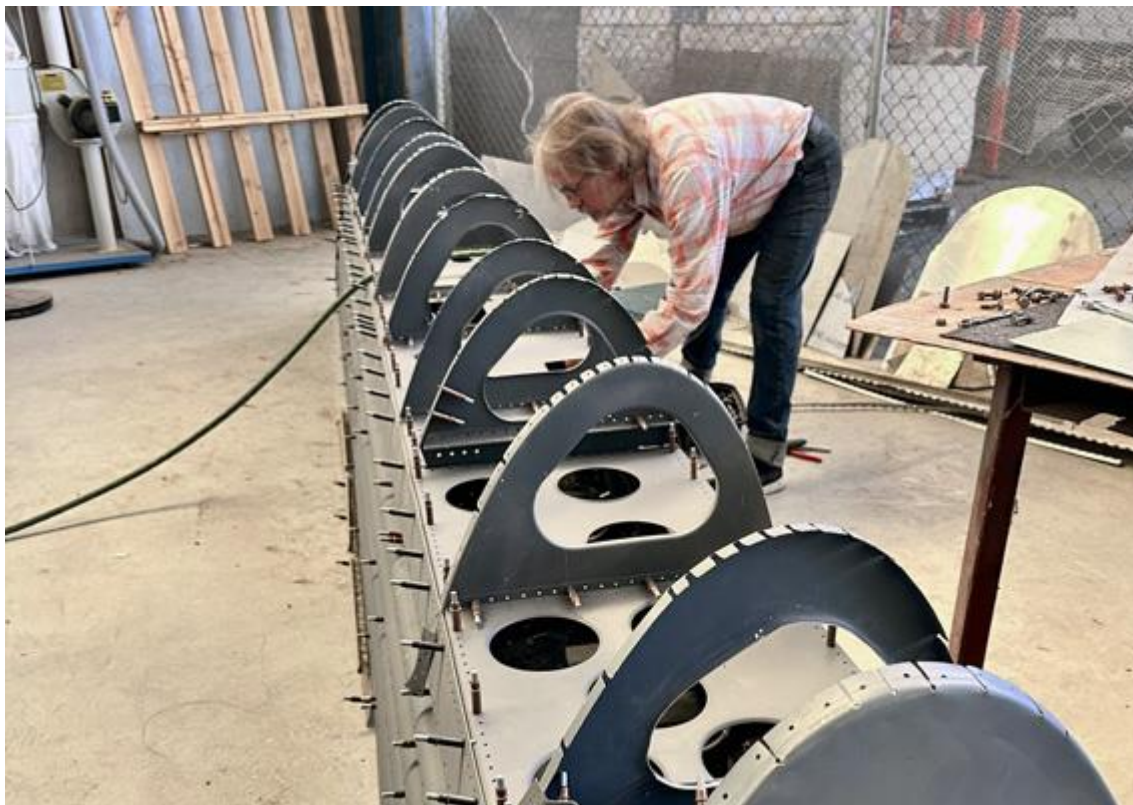
The leading edge assembly of the wing centre section nears completion.
