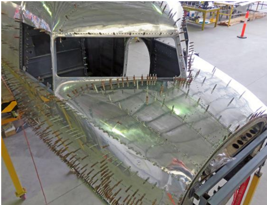
The exterior frame of the DC-2 cockpit has been completed.
