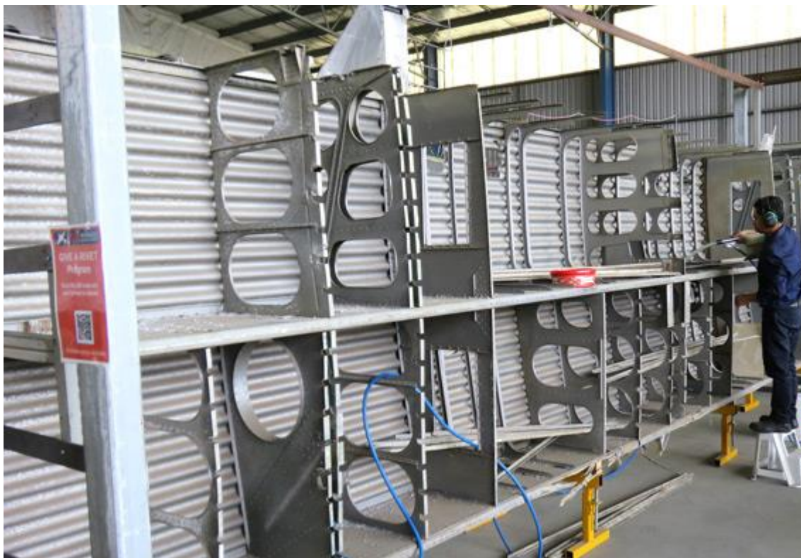
The centre wing section has been almost stripped bare.
