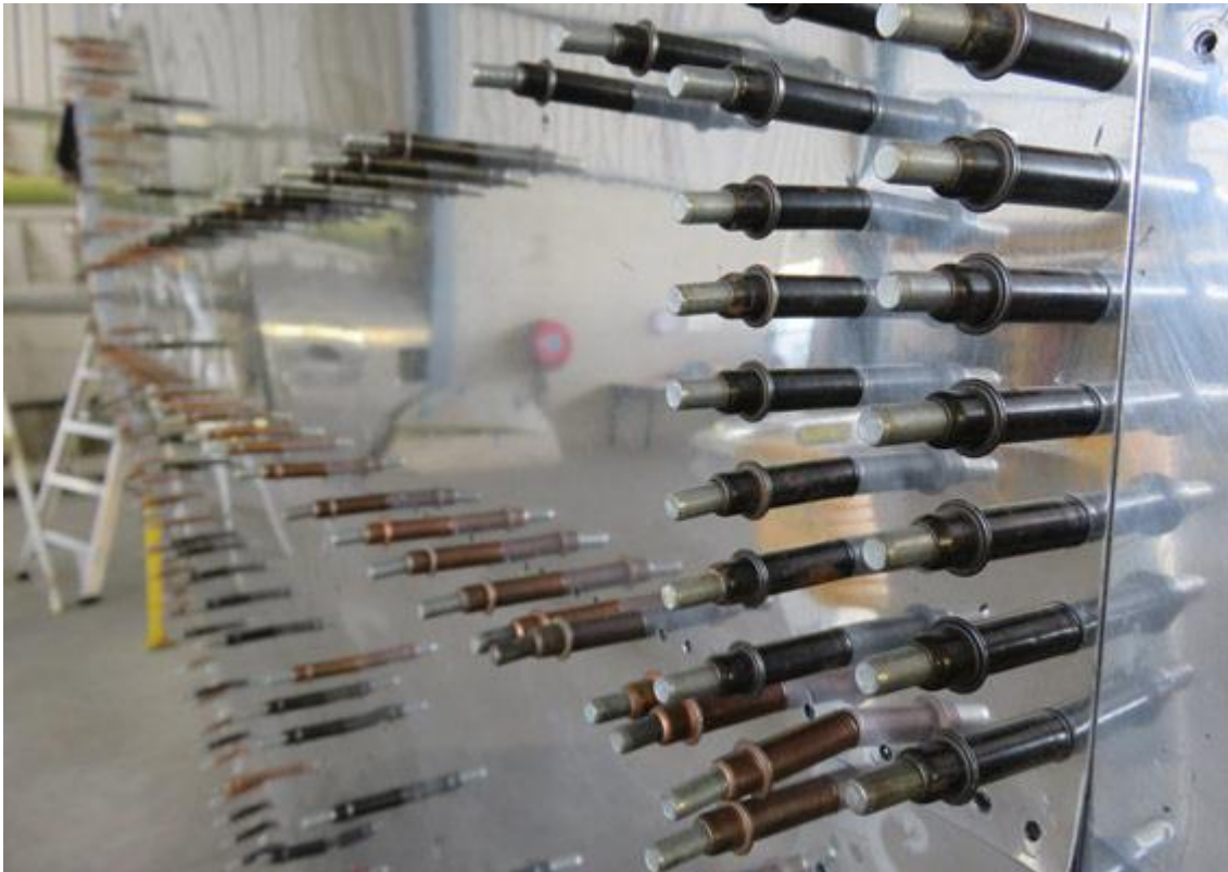
Skin pins and wing nut fasteners secure the panels in place.
