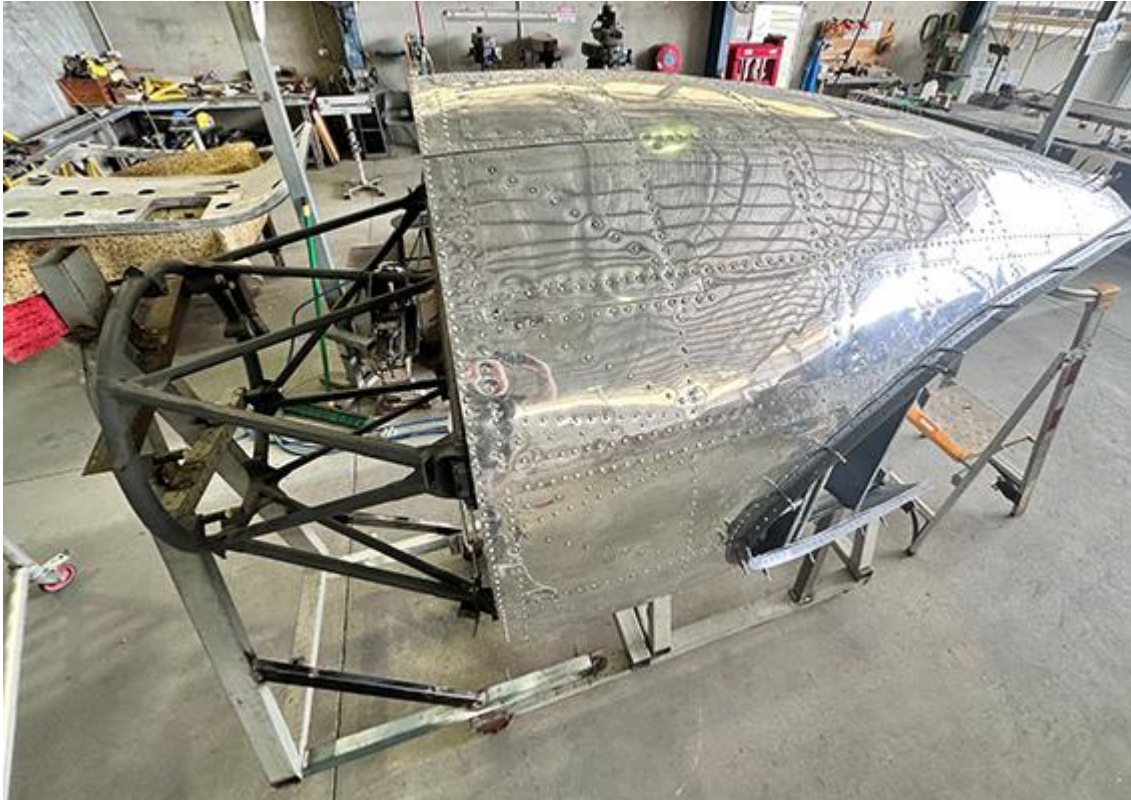
Starboard engine nacelle fully rebuilt.
