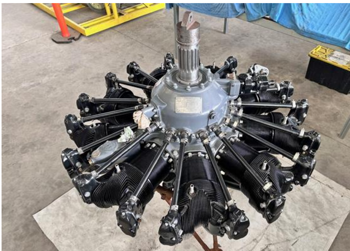
Our spare Wright Cyclone 1820 radial engine currently being restored.
